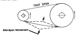
Figure 30. Drive Chain Tension
